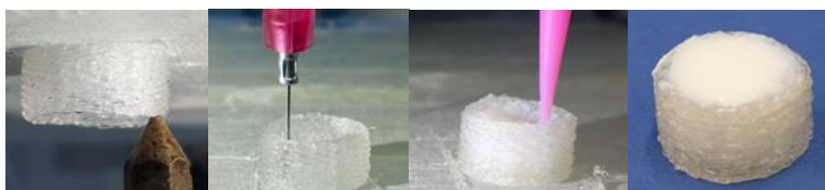
Fig. 1. From left to right: FDM extruder (PLA), IVF injecting drug-loaded gel, IVF injecting the delaying release polymer and final printfill obtained [1]
